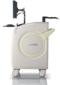
fNIRS can visualize a brain activity by measuring a change in hemoglobin volume in real time using near-infrared light.
