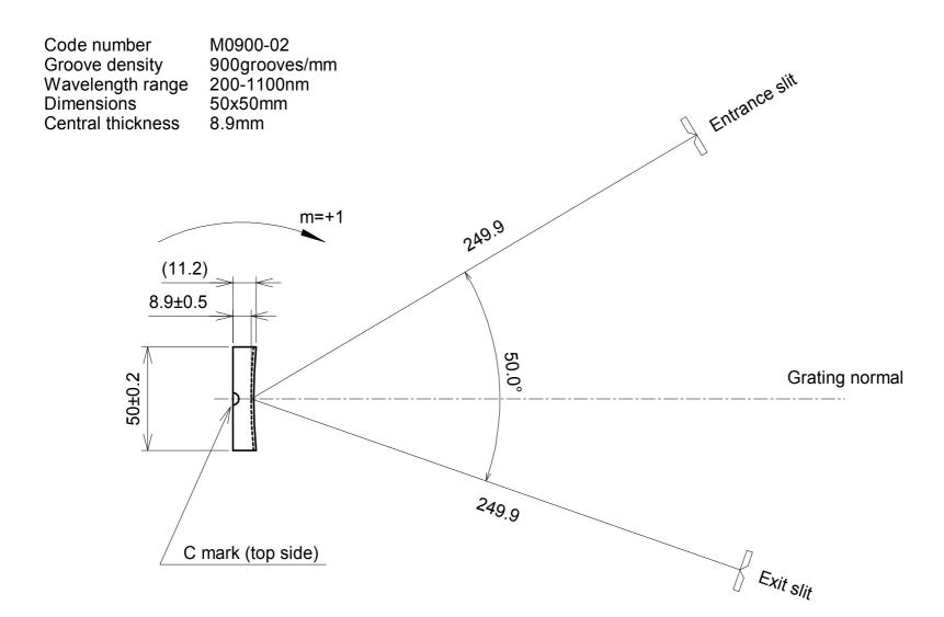
The rotation direction(arrowhead) stands for scaning direction from short to long wavelengths.
