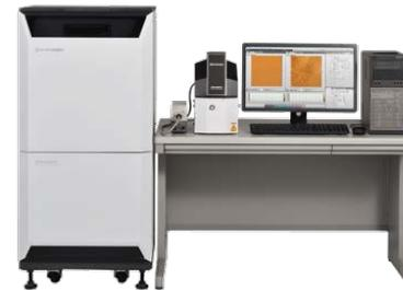
**Scanning Probe Microscopes**
