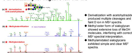
Figure 2 Negative-ion MS<sup>2</sup> spectra of in-gel derivatized A2 glycans: (a) derivatization with acetylhydrazide; (b) methylsterification; (c) methylamidation.
