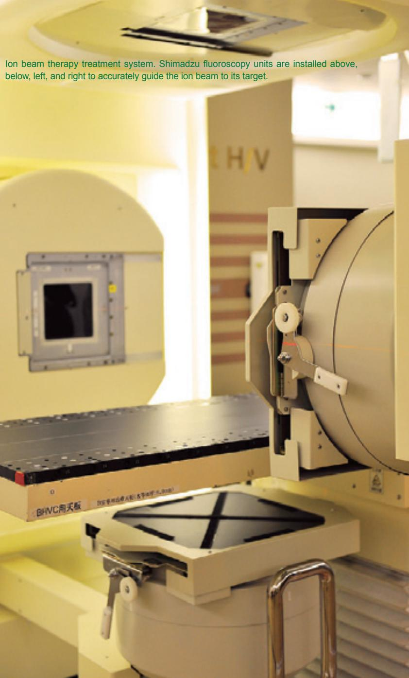
Ion beam therapy treatment system. Shimadzu fluoroscopy units are installed above, below, left, and right to accurately guide the ion beam to its target.
