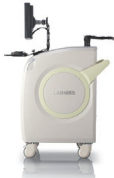
fNIRS can visualize a brain activity by measuring a change in hemoglobin volume in real time using near-infrared light.
