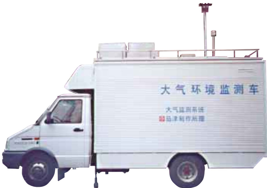
The mobile air monitoring station has become operational, with Shimadzu's monitoring system (for ambient air and meteorological parameters) and the vehicle procured and remodeled by Guiyang city.
