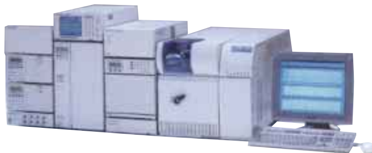
The LCMS-2010 responds to demands for trace analysis and ultra high-sensitivity analysis on complex matrices.
