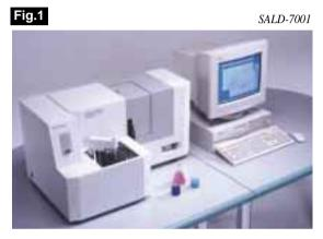
addition to determining the particle size distribution through the sub-micrometer and nanometer ranges, these measurements can detect the existence of defective particle size distributions in the micrometer and larger ranges. The SALD-7001 can truly be described as a nanotechnology device providing background support to semiconductor processing.
