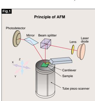
graphic image of the sample surface by tracing the minute surface shapes (X and Y axes) while providing feedback control to maintain a constant cantilever deflection (Z axis).
