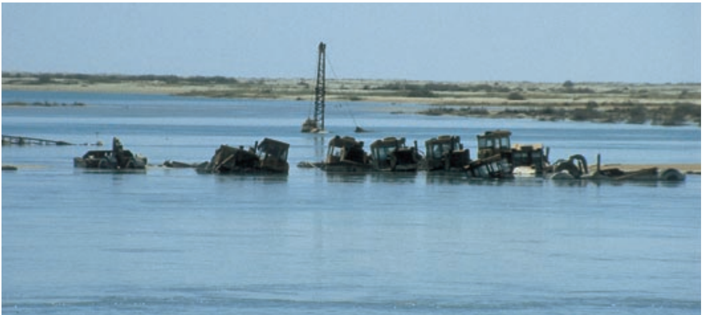
An earth dike constructed between the Small Aral and Large Aral, to protect the Small Aral, was destroyed by heavy rainfall. The accident left heavy earthmoving equipment partially submerged.
