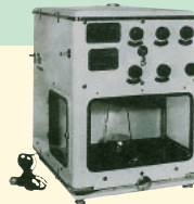
Direct reading balance "DODIC" (1950)
