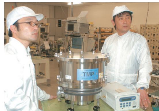
The above photograph shows a large-capacity TMP-3403LMTC turbomolecular pump being assembled in a clean room. On the right is Tatsuhiro Taguchi Asst. Manager of the Instrument Group in the Research & Development Department, and on the left is Shingo Tsutsui Asst. Manager of the Component Group.
