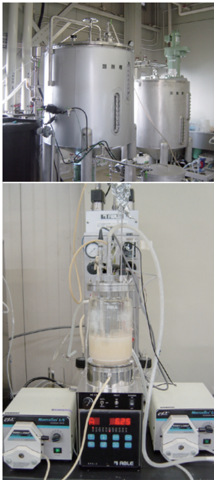
( Fig.3) 900-liter reactor <top> 1-liter prototype reactor <bottom>
