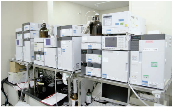
The Shimadzu High-Speed HPLC Prominence UFLC at Japan Food Research Laboratories Tama Laboratory
