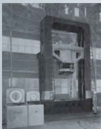
a 500-t structural member testing machine
